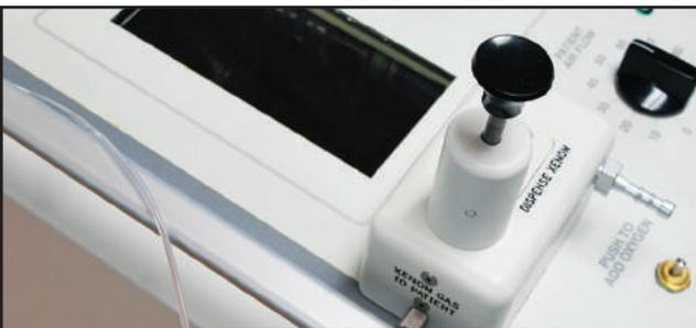
The Automatic Xenon Dispenser is easily attached to the front of the Pulmonex System without the use of tools. Preload the xenon vial into the supplied plunger. At the precise moment you want the xenon delivered to the patient, simply press the dispense button.
