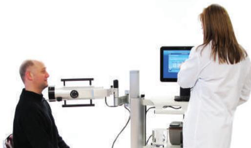
*Innovative multi-axis and height adjustable arm makes patient positioning easier than ever before. Combined with unique Positioning LED and Distance Measurement Rod, the Atomlab 960 allows for repeatability in uptake measurements.*
