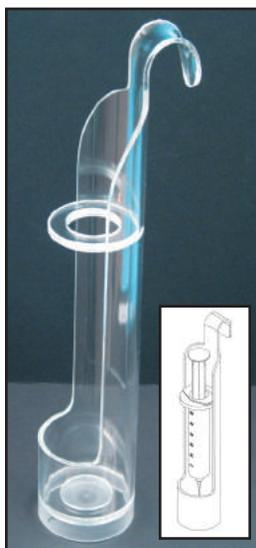
The Syringe Dipper will hold a 60 cc syringe in the correct position in most commercial dose calibrators with 2.5" x 10" well chamber interior. The material used will not cause attenuation problems and is very resistant to breaking.
