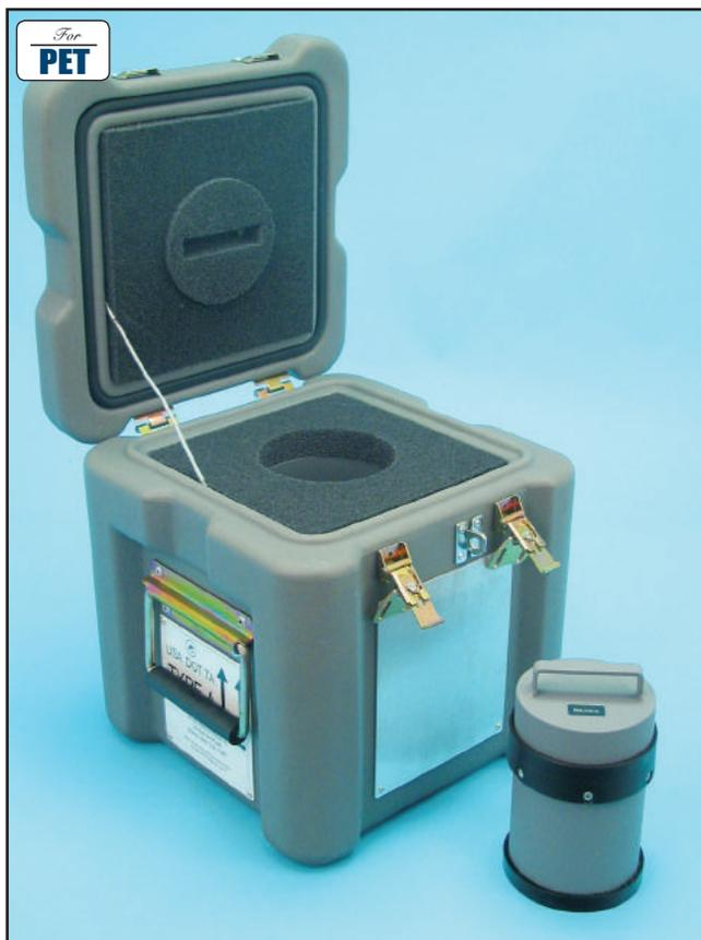
Transport up to a 30 ml vial of PET pharmaceutical in the PET Shipping System. The complete system offers 1.55" lead shielding to accommodate 1.5 curies of FDG F-18 and meets DOT II Type A packaging requirements.
