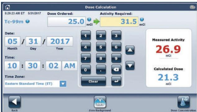
The Atomlab 500 Dose Calibrator features a nuclear pharmacy “Dose Calculation Screen” to meet the needs of a commercial nuclear pharmacy. All the information needed to draw doses efficiently is readily available on one screen. The feature easily performs pre- and post-decay calculations, volume calculations for specific times and isotope changes all with minimal screen touches. No calculators needed!
