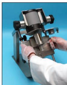
*Syringe is placed in the Dose Drawing Syringe Shield. The vial shield rotates to 45-degree downward angle. Swing open the cover for vial septum access.*
