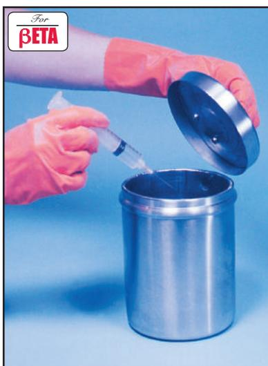
*Eliminate clutter and reduce safety hazards with convenient Shielded Storage Containers*
