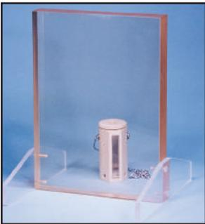
**T**he Bench Top Shield for gamma radiation is constructed of 1.375" thick (35 mm) lead acrylic, providing the equivalent of 0.060" (1.5 mm) lead for shielding gamma radiation. Lead acrylic can be used with low-energy gamma emitters. Lead acrylic is not recommended for beta emitters. This lightweight, sturdy shield is ideal for use in hoods, on laboratory benches or any "hot" area where local shielding is needed.
