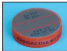
Instrument functionality is easily assessed with a Cs-137 Check Source. The activity is 10  $\mu\text{Ci}$ . No license is necessary.
