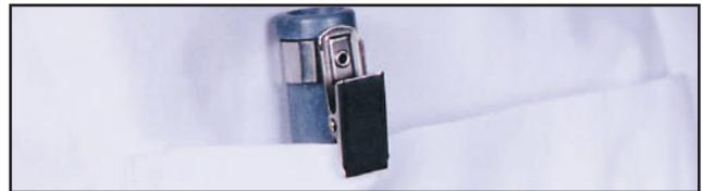
For personnel working in radiation areas, Direct Reading Dosimeters provide an accurate and instantaneous indication of accumulated exposure.
