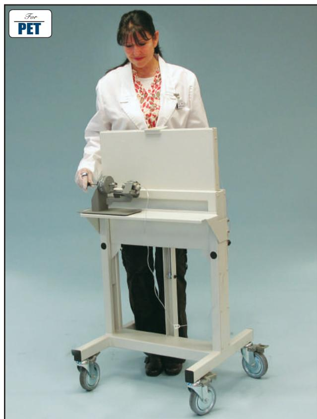
The Compact Adjustable Height Radiation Shield is a versatile addition to any PET site. The 1" thick lead panel is 22" w x 19" h. The panel can be height adjusted within a 10" range. The shield can be used to protect technologists from sitting or lying "hot" patients. A fold down shelf is conveniently located to hold syringe shields, carriers and injectors, etc. Place shielding where and when it is needed. Wheel and swivel locks on each caster provide secure placement.
