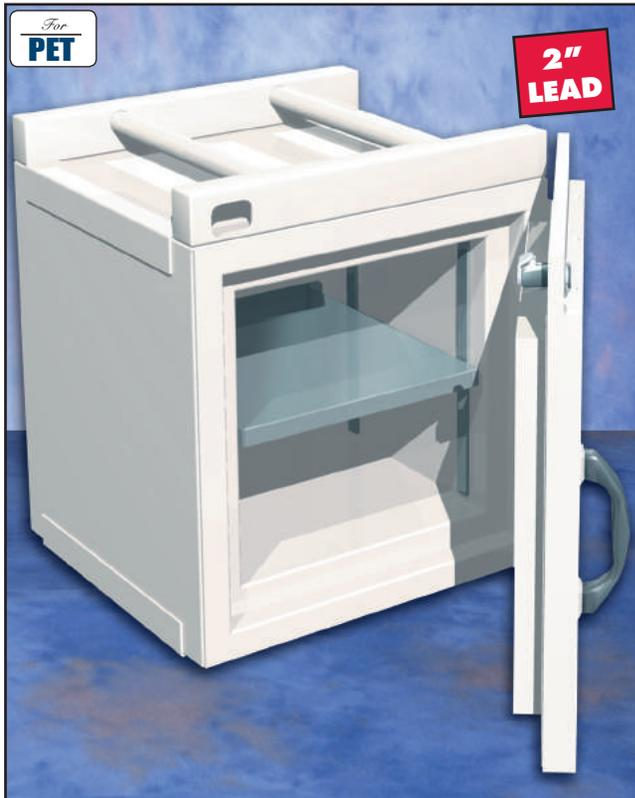
Conveniently loaded from the front, this Storage Safe is ideal for storing large quantities of high-activity radioisotopes. Shielded with a thickness of 2" of lead, the safe is encased in a powder-coated steel jacket and features an adjustable shelf. The lead-lined door is hung with heavy duty non-sagging hinges and is key-locked to prevent unauthorized access.
