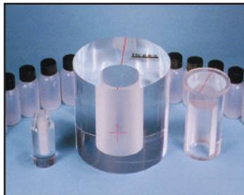
**T**he Neck Phantom is designed to simulate a patient's neck. The phantom is constructed of lucite. It has a two part insert that allows counting from a bottle, vial or capsule. A capsule holder is supplied to enable the user
