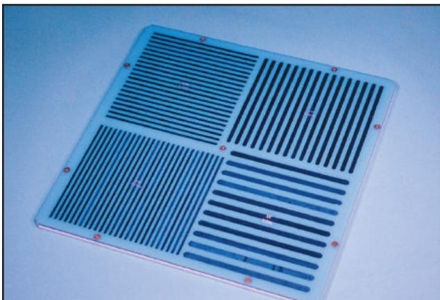
**F**our-quadrant Bar Phantoms offer precise determination of camera intrinsic resolution, collimator spatial resolution, field size and linearity. We offer a range of sizes manufactured to the highest quality standards.
