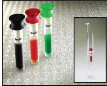
The daily calibration of your dose calibrator is recommended to ensure accurate and reproducible instrument response. Calibration, using long-lived standards, should be performed in a manner that most closely represents
