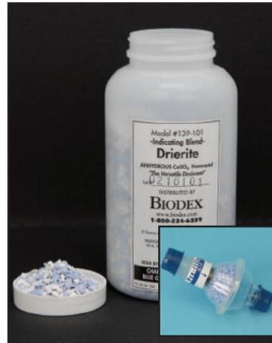
Drierite serves as a moisture trap for the air going into the charcoal trap of the Pulmonex Xenon System. Drierite is blue and white when dry and turns pink when it has absorbed maximum moisture. Available in two convenient sizes, Drierite is packaged in an air-tight container with a wide-access mouth.
