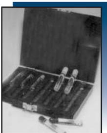
To calibrate well type scintillation crystals, Biodex offers a variety of Rod Sources to meet department needs. You can count on consistent accuracy. Rod Sources are calibrated as NIST traceable with an accuracy of  $\pm 5\%$  at the 95% confidence level.
