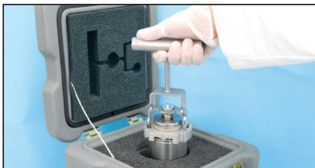
The Vial Shipping System employs a unique Tungsten Vial Shield for use with the Medrad® Intego™ PET Infusion System. Manufactured to Medrad's specifications, the Vial Shield transports a 30 ml Hospira vial.
