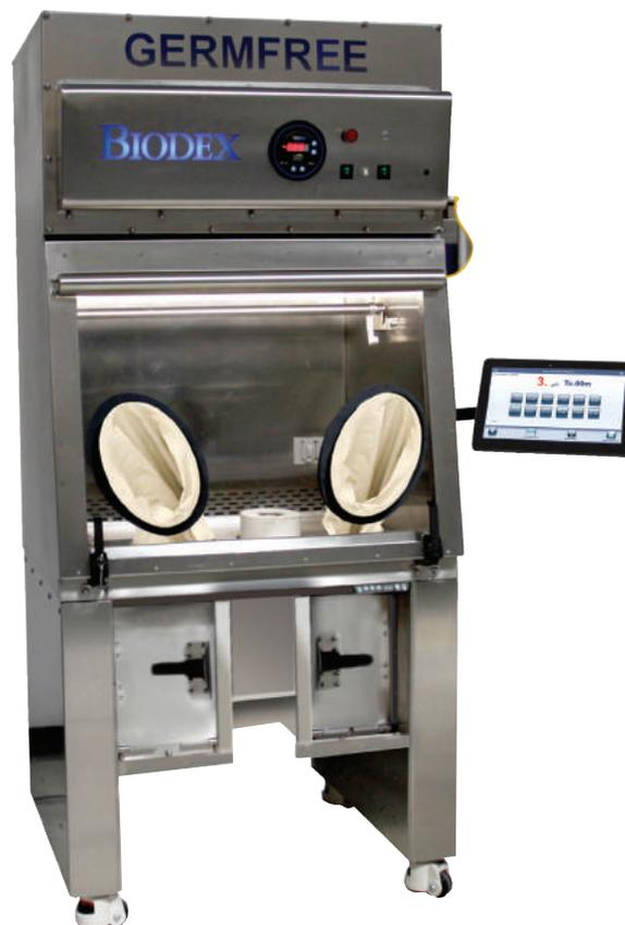
a ISO Class 5 (Class 100) environment for product preparation, with work occurring inside a closed, pressurized environment accessible only via sealed gloves that reach into the work area.
