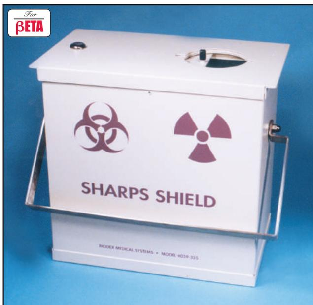
**T**his Sharps Container Shield is a simple way to dispose of used syringes that may be contaminated with low-energy gamma and beta radiation residue. The shield is constructed of steel, lined with .125" lead and .0625" aluminum. The shielding combination attenuates gamma radiation, beta radiation and errant bremsstrahlung.
