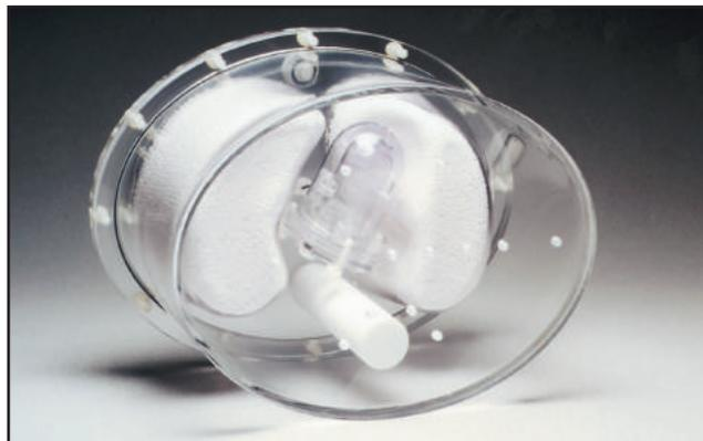
Lung-Spine Phantom shown with Cardiac Insert in place and Elliptical Cylinder
