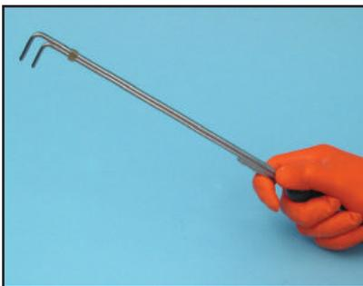
**T**hese low-cost tongs are used to handle small radioactive or otherwise dangerous objects up to 1" diameter. The tongs have a 45° v cut groove on each jaw. The compression spring maintains a strong grip on the object until the tension is released by
