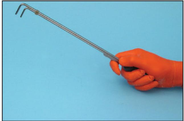
**T**hese low-cost tongs are used to handle small radioactive or otherwise dangerous objects up to 1" diameter. The tongs have a 45° v cut groove on each jaw. The compression spring maintains a strong grip on the object until the tension is released by squeezing the finger bar. Niptongs are made of chrome-plated, high carbon steel with hardwood handles and are easily disassembled for decontamination and cleaning.
