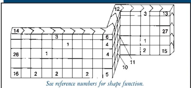
*This wall demonstrates the dimensions and alternative positions of all variations of the standard brick wall. The walls should be built with male chevrons directed upwards and to the right, as viewed from the outside of the cell.*
