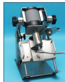
*Syringe shield slides upward, allowing the syringe to puncture the vial septum. Dose is drawn.*
