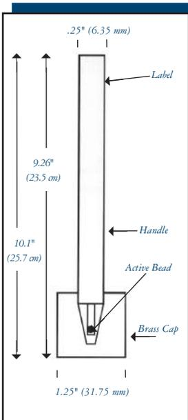
The Pen Point Marker Source contains Co-57 in a ceramic matrix at the end of a 9.26" (23.5 cm) anodized aluminum rod. The pen-shaped rod screws into a brass cap which shields the active point. The Pen Point Marker Source is used in tracing the outlines of anatomical features on a patient. The trace appears almost instantly on the camera display. Contained activity is supplied as a nominal value  $\pm 15\%$ .
