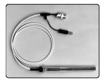
CT Dose Probes to calculate CT Dose Index 3.2 cc volume over 10 cm length Calibrated in units of R•cm/ Coulomb
