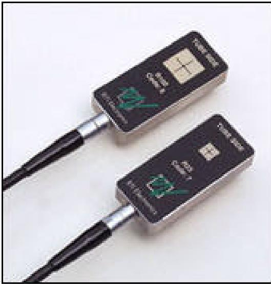
The R25 and R100 can be used for film and skin dose, dose rate to image intensifier, mAs linearity, HVL, reproducibility, HVL, and AEC measurements.
