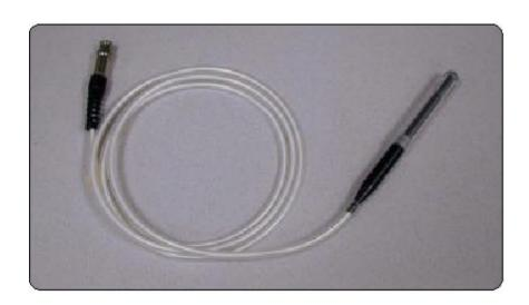
Stable, reproducible absolute dosimetry measurements In-air calibration of brachytherapy sources Precision machined thimble for flat energy response Hemispherical electrode design, no electrical field distortion Rugged **replaceable** PMMA thimble, 0.5 mm thick Non-waterproof version available, Model 580-006
